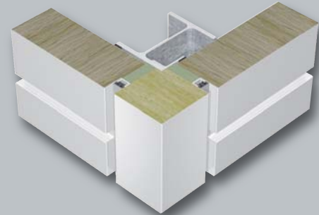
Corner design without continuous joint
